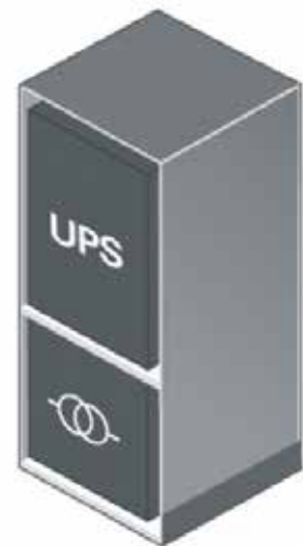
UPS with isolation transformer
